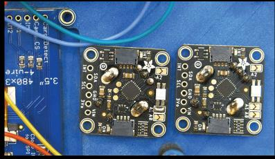
Wire up the two switches to ground, power and pins 24 and 25 on the feather. Trim off any loose wires off of the back of the circuit board, and secure it in place with a few blobs of hot glue.
