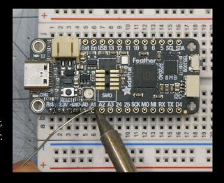
Next we'll need to set up our solder-type breadboard. This is a board that we can use to connect all of our components to the Feather. It has built-in connections for each row on the circuit board. We also need to create a power and ground rail using this board. Place the Feather into the board. The board is much larger than we need, so you can cut down the board to the size you see here.
