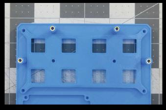
Place the Key Switch Mounting plate as you see in the above photo. Attach it in the four outermost corners using four 8mm m3 screws. Flip the part over and insert the key switches. I'm using RGB Cherry MX Blue Switches, but the important thing is that you align the switches correctly. The pins should be at the top and the LED window at the bottom. Snap all eight of them into place.
