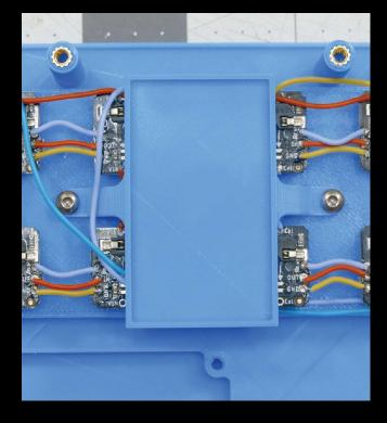
Use a 3rd hand tool to hold the feather just above the 3d printed feather mount. While it's suspended in place, trim each of the connecting wires for the screen and key matrix, and then solder them to their corresponding pins on the breadboard. Refer to the provided wiring diagrams so see where everything should connect to the Feather RP 2040.
