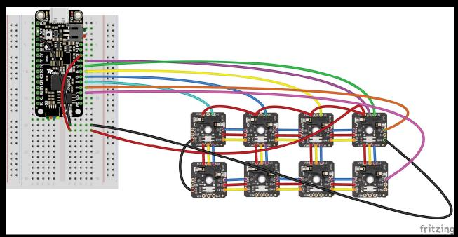
Solder two rotary encoders to the two Stemma QT rotary encoder breakouts. On only one of them, place some solder across the A1 solder pad. This will make sure they have different i2c addresses.
