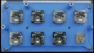
Once they're all apart, we need to solder them back together. Snap them into place on the pins of the key switches. You'll need to re-solder the wire connections, both horizontally and vertically between each key pad. You'll also need to connect each of the ViN connections along the top row, and the ground connections on the left side. This will take a while. Be patient, listen to a good audio book and take your time.
