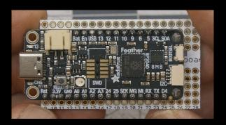
Note which rows the Ground and USB pins connect to. We'll need to solder on some wires that will connect these rows to a power and ground rail towards the bottom of the board. These wires will be underneath the board once it's soldered in place, and won't be accessible afterwards, so make sure they're lined up correctly before soldering. Trim off the header pins so they're flush with the underside of the board.
