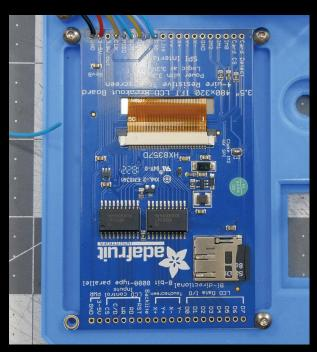
Attach the screen to the enclosure top using 6mm M3 screws, making sure your soldered connections are facing upwards.
